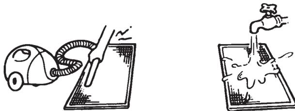
Use a vacuum cleaner A) or wash the air filter with water B).
